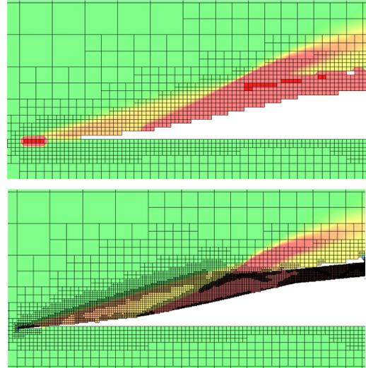
Figure 2. Progressive Mesh Adaptation Cycle 0 [top] and 8 [bottom]
