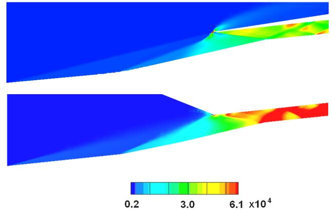
Figure 3. Cart3D [top] and CFD++ [bottom] Pressure Contours (Pascals)
