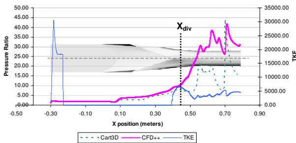
Figure 5. Mach 4.5 static pressure comparison between viscous and inviscid solvers  $\alpha=0^0, \beta=0^0$
