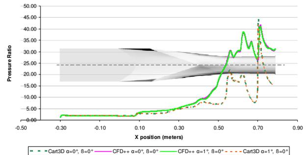
Figure 6. Mach 4.5 static pressure comparison between viscous and inviscid solvers  $\alpha=0^0, \beta=0^0$
