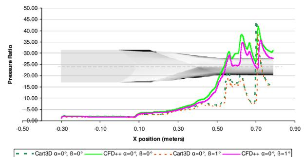
Figure 7. Mach 4.5 static pressure comparison between viscous and inviscid solvers  $\alpha=0^0, \beta=1^0$
