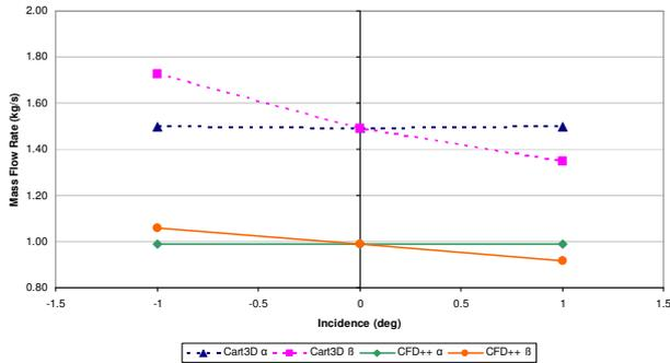
Figure 8. Mass Flow Rate at end of isolator comparison
